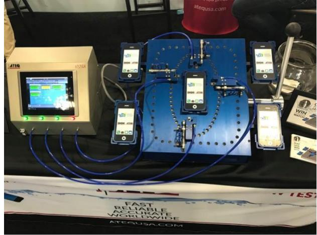
ATEQ's leak testers use pressure decay air leak testing to measure pressure drops, which determine the air leak rates within the device. There is a certain relative air to water correlation ratio that can be used to essentially say, "if only a miniscule 'x' amount of air can leak in or out of the device, then the device is waterproof", since air molecules are much smaller than water molecules.
